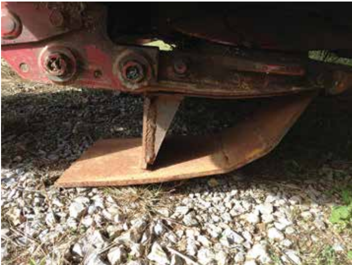
Figure 5. Example of a fabricated skid shoe that allows for increased cutterbar height.
