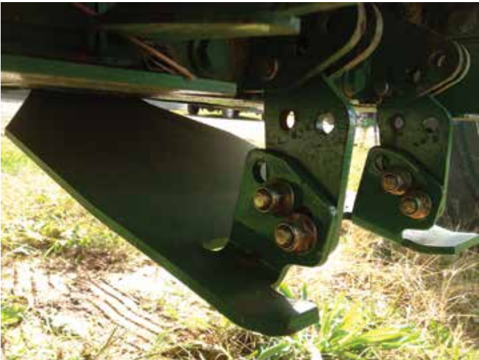
Figure 7. Skid shoe spacers, installed on a 600-series John Deere mower-conditioner, provide additional lift for the cutterbar and greater residual heights.
