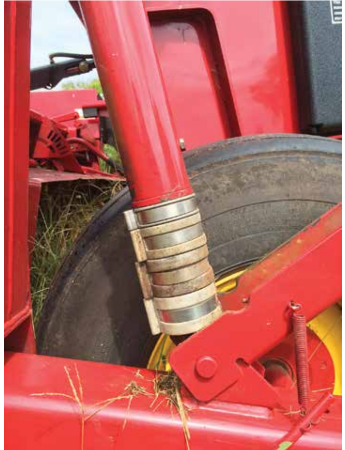
Figure 3. Stroke-limiting collars installed on mower-conditioner lift cylinders can be used to raise cutterbar height.
