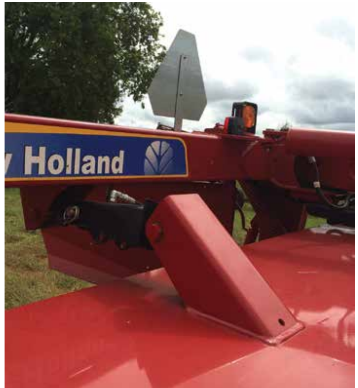
Figure 8. Cutterbar angle can be adjusted as seen here on a New Holland mower-conditioner.
